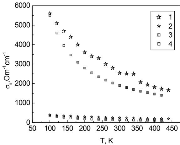
Fig.2. Temperature dependencies of the components of electrical conductivity tensor  $\sigma_{ij}$ : 1( $\sigma_{11}$ ), 2( $\sigma_{33}$ ) – experimental; 3( $\sigma_{11}$ ), 4( $\sigma_{33}$ )-calculated according to double-band model
