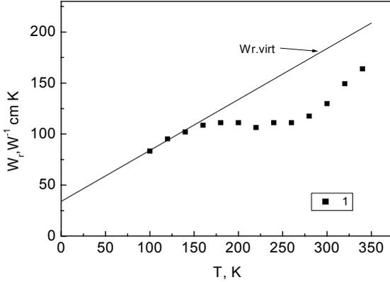
Fig.4. Temperature dependencies of lattice thermal resistivity ( $W_r=1/\kappa_{r11}$ ): 1- calculated according to single-band model
