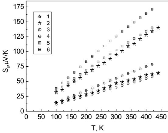
Fig.1. Temperature dependencies of Seebeck coefficient tensor  $S_{ij}$ : 1( $S_{11}$ ), 2( $S_{33}$ ) – experimental; (3-6)- calculated values; (3,4) at  $r=0$ ; 5,6 – at  $r=2$ ; (1,3,5) – along the cleavage plane; (2,4,6) – along a trigonal axis  $C_3$
