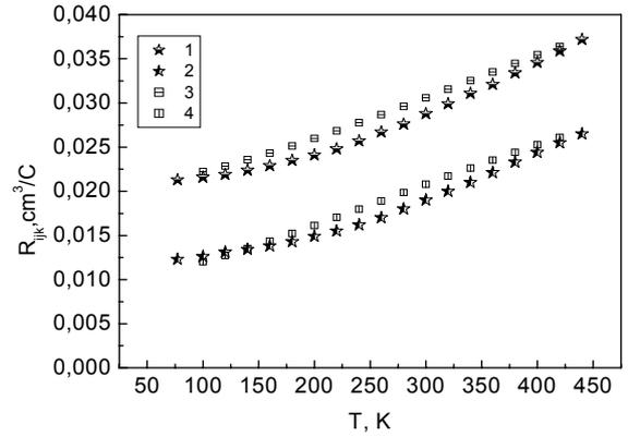
Fig.3. Temperature dependencies of the components of Hall coefficient tensor  $R_{ij}$ : 1,2 – experimental; 3,4 – calculated according to double-band model (1,3 –  $R_{123}$  – magnetic field (H) is parallel to  $C_3$  trigonal axis; 2,4 –  $R_{231}$  – H is perpendicular to  $C_3$  axis)
