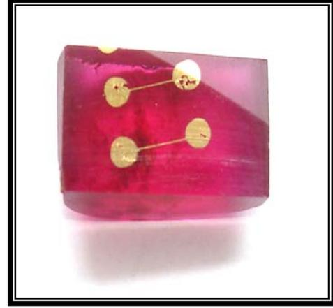
Fig.4 Ruby single crystal with the deposited strips of gold.
